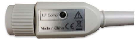
Figure 2. Low-frequency compensation adjustment (for N2840A/41A/42A/43A/53A)
