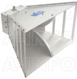
LB-660-NF Broadband Horn Antenna 0.6-6.0 GHz 11dB Gain N Type Female
