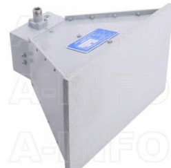
LB-1080-NFSPO Broadband Horn Antenna 1-8GHz 11dB Gain N Type Female
